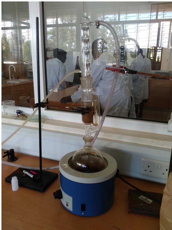
Figure 5: Preparation of stem bark extract of Acacia nilotica under Soxhlet apparatus
