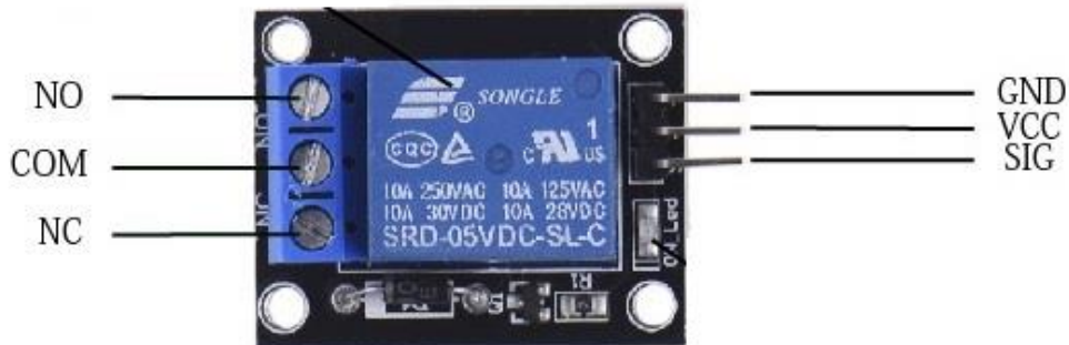
Figure 28: Pin configuration of a single channel relay module
