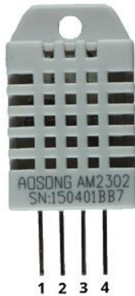
Figure 27: Digital humidity and temperature sensor 22 pinouts
