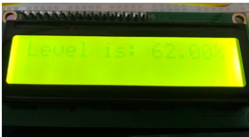
Figure 32: LCD displays percentage level of juice
