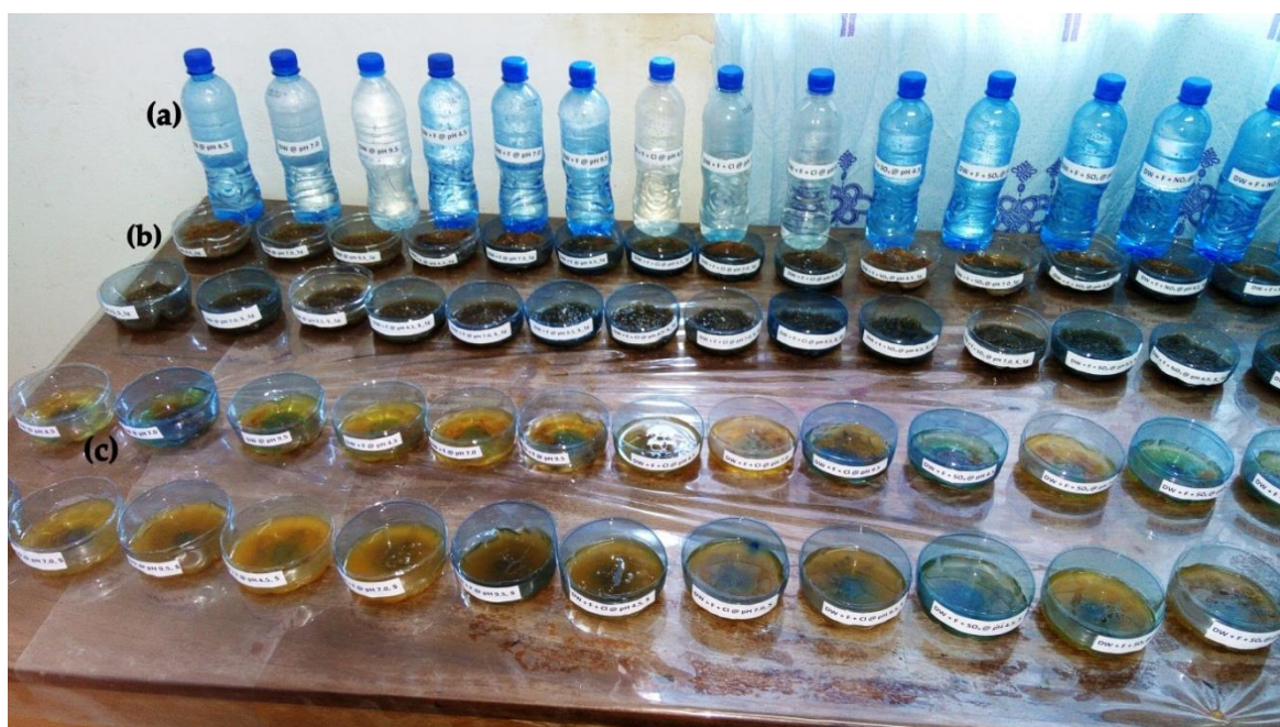
Plate 1: An optical picture of the actual laboratory set-up showing, from left to right, the (a) prepared samples (b) corroded 1.0 g of SW in non-disturbed (first row) and disturbed (second row), and (c) corroded 0.1 g of SW in non-disturbed (first row) and disturbed (second row)
