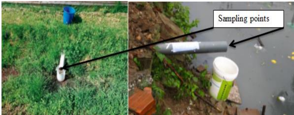
Figure 8: Sampling point of a septic tank effluent at soakaway pit
