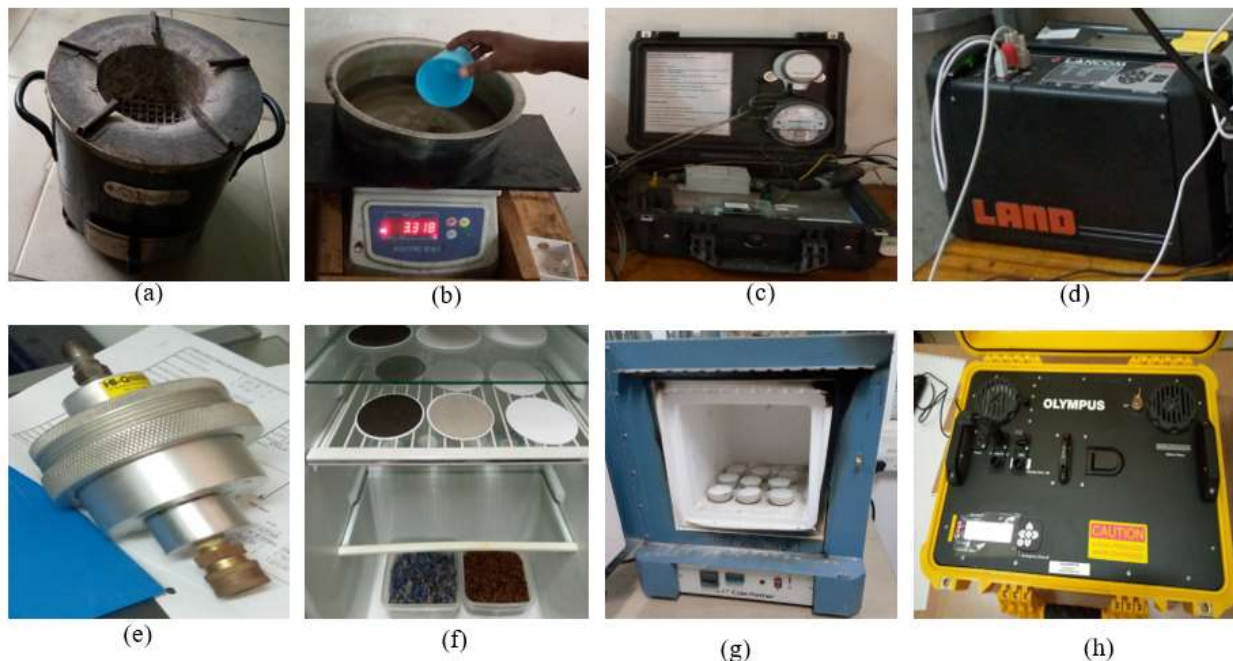
Figure 19: (a) Cookstove (Burn), (b) Weighing water, (c) gas analyser (PEMS, 2000) , (d) gas analyser (Ametek Land, lancom 4), (e) Filter holder, (f) Drying the filter paper, (g) furnace, (h) XRD/XRF analyser
