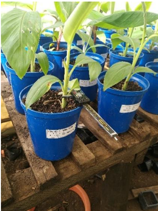
Appendix 15: Determining plant girth using digital caliper (Source: This study)
