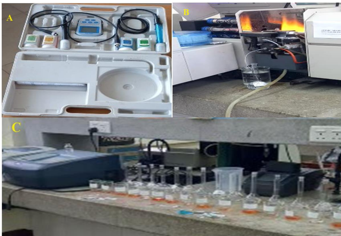
Plate 2: Instruments used in measuring the physicochemical water quality parameters and analysis of the heavy metal concentrations. A – Multiparameter (40HQd), B – Atomic Absorption Spectrophotometer (AAS), C – Hach spectrophotometer (DR6000)
