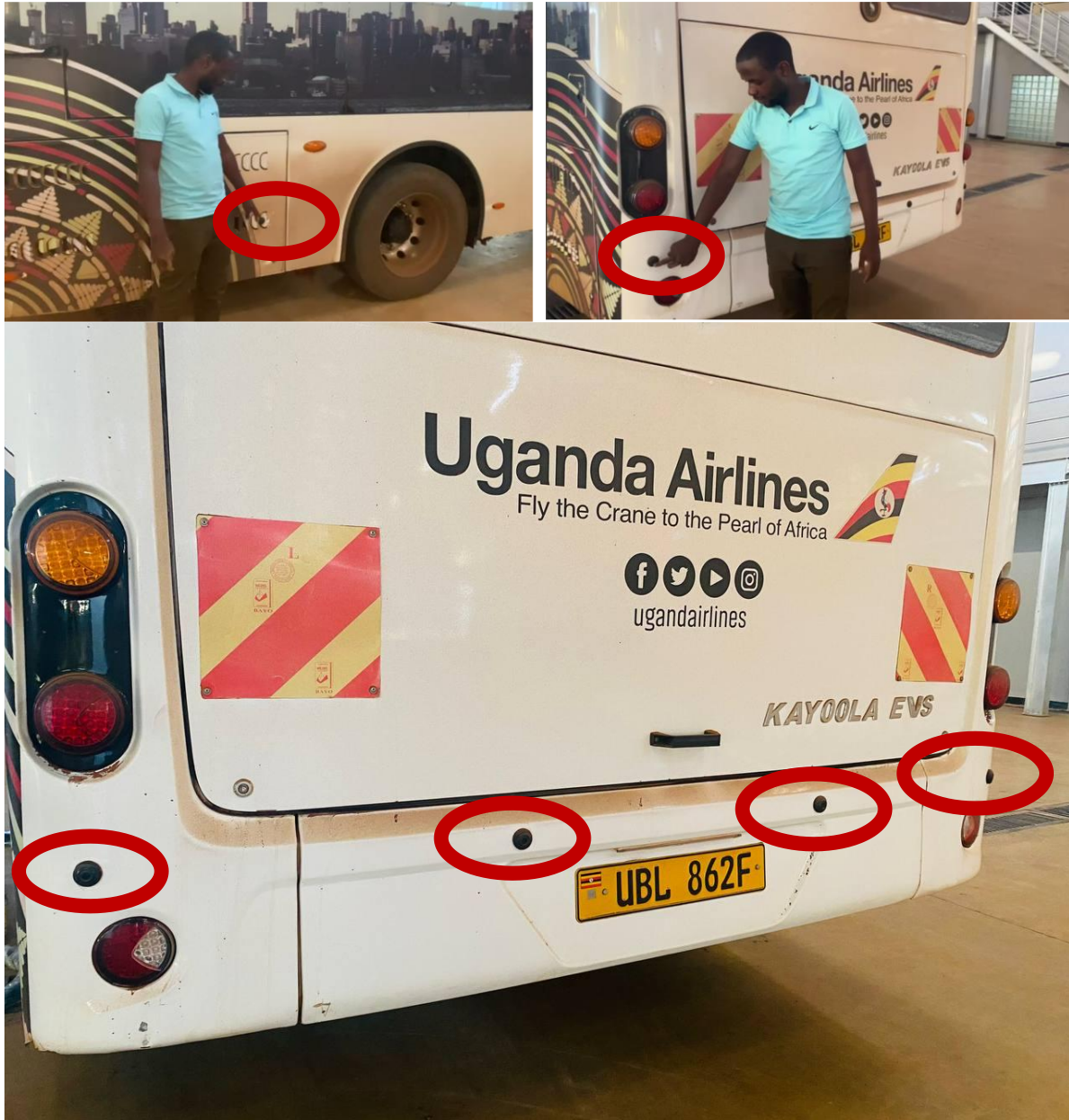
Figure 25: Integration of proximity sensors
