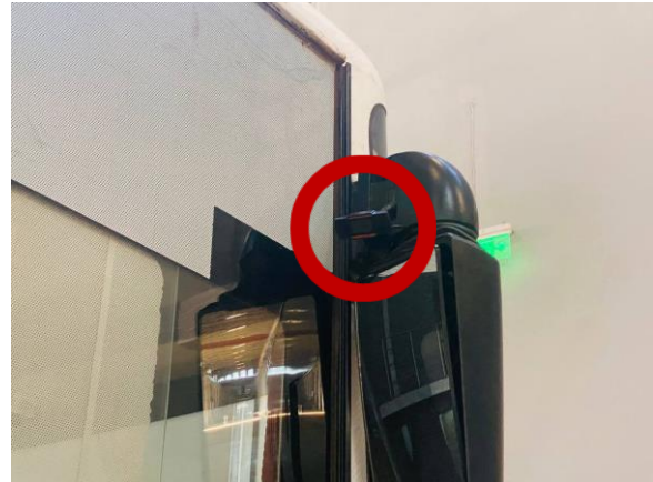
Figure 23: Installation of the right and left-hand side cameras
