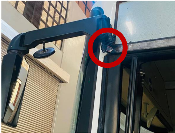
Figure 23: Installation of the right and left-hand side cameras
