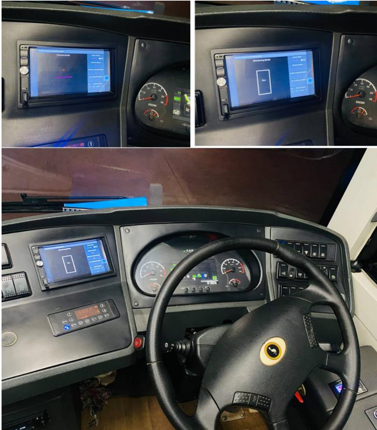
Figure 27: Integration of the display in the Kayoola EVS Bus
