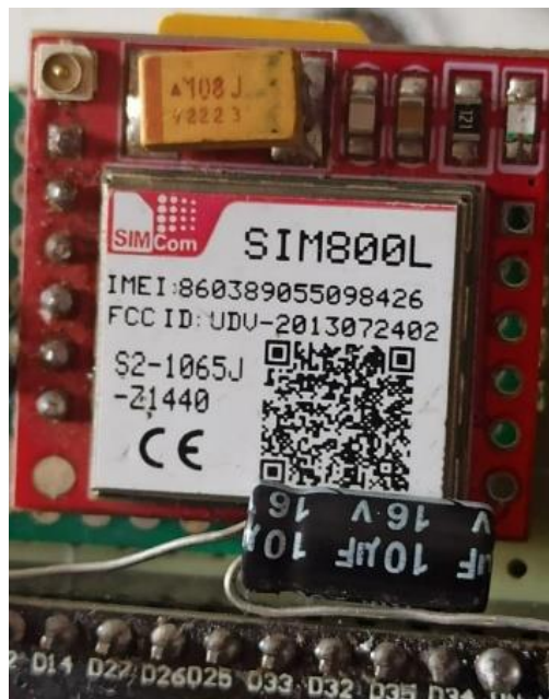
Figure 28: The SIM800L GSM Module
