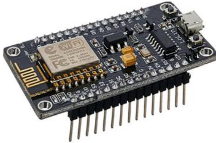
Figure 21: The DOIT ESP32 DevKit (Cameron, 2023)
