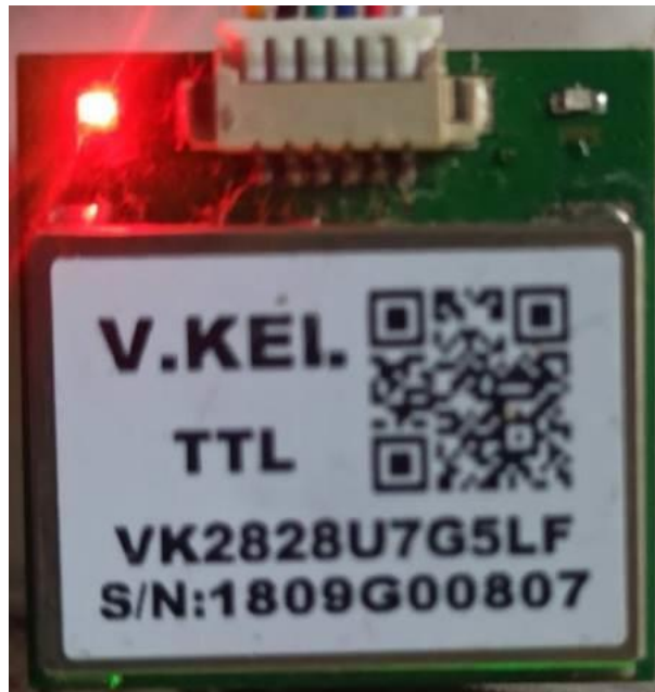
Figure 26: The V.KEI GPS Module
