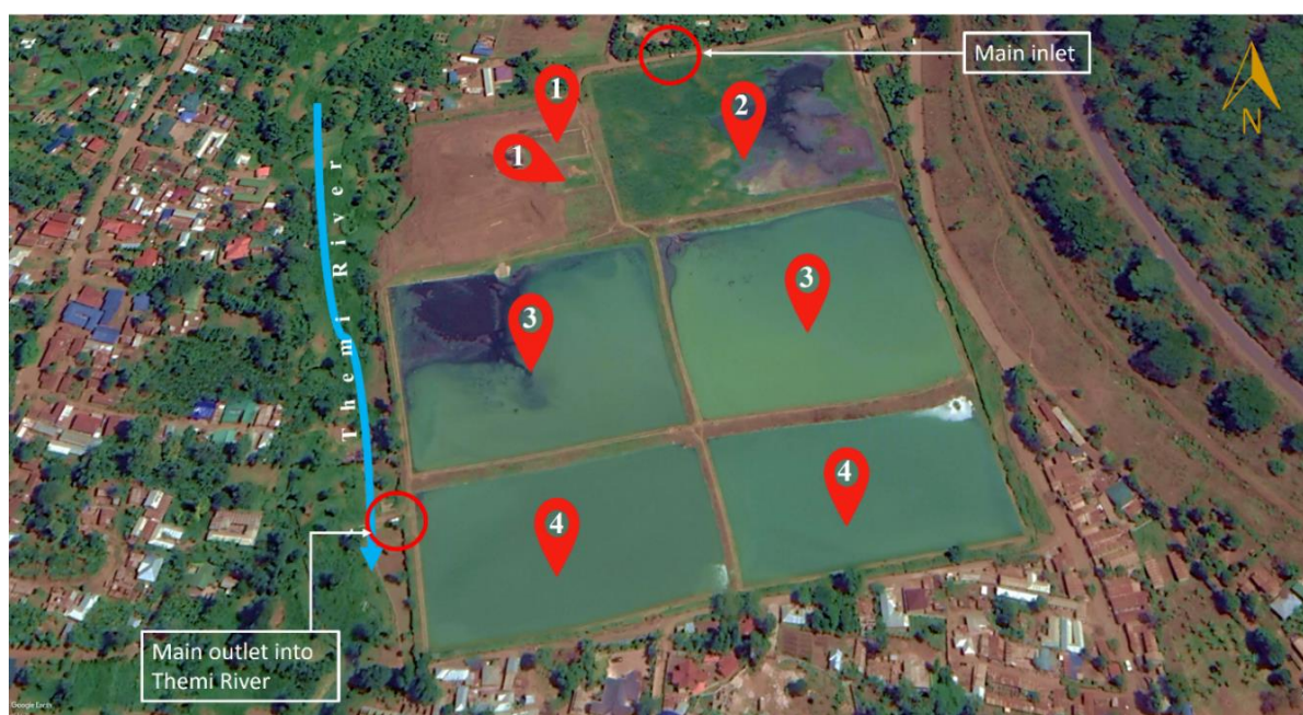
Figure 1. Layout of Arusha waste stabilisation ponds from Google Earth TM : Blue arrow line on the left indicates the direction of flow of Thembi River. Placeholder 1 = Domestic wastewater disposal tanks, 2 = Anaerobic pond, 3 = Facultative ponds, and 4 = Maturation ponds.
